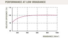
Typical module performance under low irradiance conditions in comparison to STC conditions (25  $^{\circ}\text{C},~1000\,\text{W/m}^2\text{)}.$
